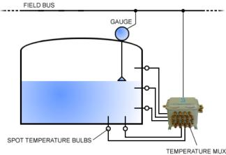
TEMPERATURE MUX AND TRANSMITTER
