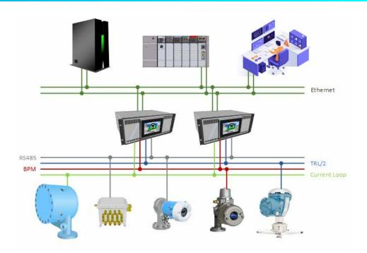
The Mini Receiver has 2 Ethernet ports, which can be configured to support redundant Ethernet or as separate networks. Devices in a redundant configuration may either use one of these ports to synchronise themselves, or a pair of serial ports. The performance of the Mini Receiver can be monitored via a built in SNMP interface allowing access to statistics such as the number of communication faults on a field bus, when and why redundant switchovers have occurred
